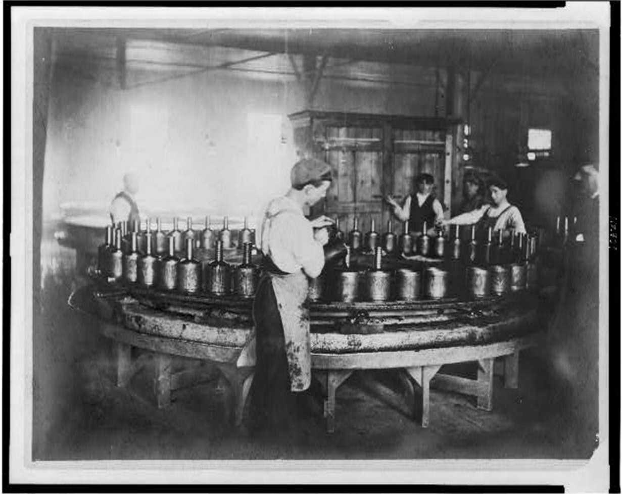
Image 5: Photographer unknown, photograph of boys working, Boys pouring wax (?) into molds in factory , c.1902. Public domain. Library of Congress, Prints & Photographs Division. http://www.loc.gov/pictures/item/95502045/ .
